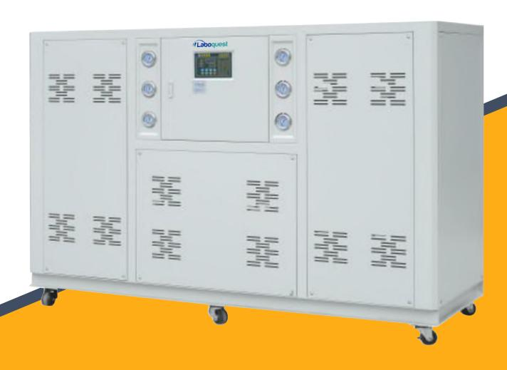
Water cooled chiller WCQ 2000 is a micro-computer controlled chillers with a temperature range from 3 °C to 30 °C. It is equipped with a refrigerant type of R134A / R22 / R407C / R410A / R404A. It has a refrigeration capacity from 8251 kcal/h to 170383 kcal/h. It is equipped with a hermetic scroll type compressor which prevents leakage.
